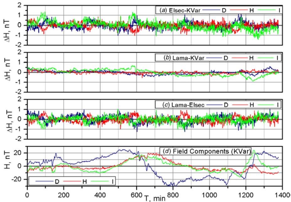
**Figure 5.** 24 h record, 1 December 1999. Reading differences between (a) Elsec8200 and K-variometer, (b) Lama fluxgate and K-variometer, (c) Lama fluxgate and Elsec8200 and (d) the Earth's magnetic field components measured by K-variometer. Notation here and after: D—field declination, I—field inclination, H—field scalar value; KVar—K-variometer, Elsec—Elsec8200 variometer, Lama—Lama fluxgate.
