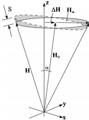
Figure 1. General principles of the vector variometer.
