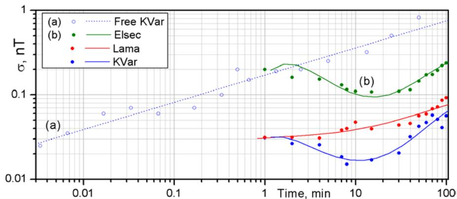
**Figure 6.** (a) Free KVar—Allan variance of stand-alone K-variometer readings in the Earth's magnetic field; (b) Allan variances of K-variometer, Elsec8200 and Lama fluxgate calculated from their reading differences (figure 5)-declination channel: KVar—K-variometer, Elsec—Elsec8200 variometer, Lama—Lama fluxgate.
