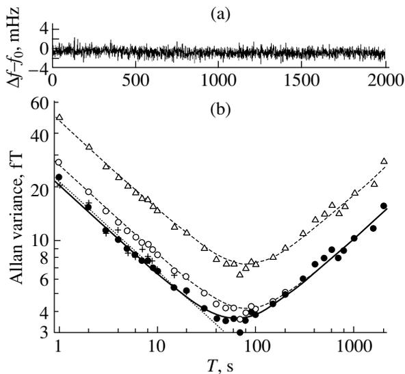
**Fig. 5.** (a) Record of the difference frequency  $\Delta f = (3f_{85} - 2f_{87})$ ,  $f_0 = 12.868$  Hz; (b) (○) Allan variance of the difference frequency  $\Delta f$ , (○) Allan variance of the frequency  $f_{87}$  (including the measuring system noise), (●) Allan variance of the frequency  $f_{87}$  (the measuring system noise subtracted), and (+) sensitivity of the  $^{87}\text{Rb}$  channel that is found from the resonance steepness-to-shot noise ratio.
