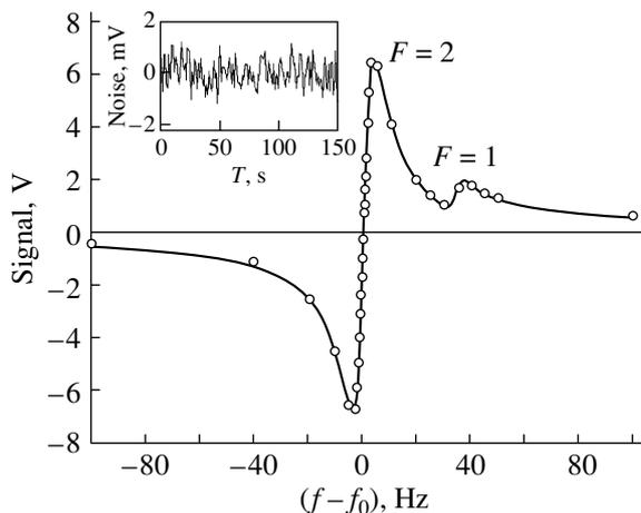
**Fig. 4.** Resonance line of  $^{87}\text{Rb}$  versus the shot noise of the photocurrent ( $\tau = 1$  s).  $\Gamma(\text{HWHM}) = 3.74$  Hz,  $f_0 = 8192$  Hz,  $dS/df = 3.33$  V/Hz,  $\sigma_{87}^{\text{light}} = 21.5$  fT s $^{1/2} = 53.7 \pm 2$  fT Hz $^{-1/2}$ .
