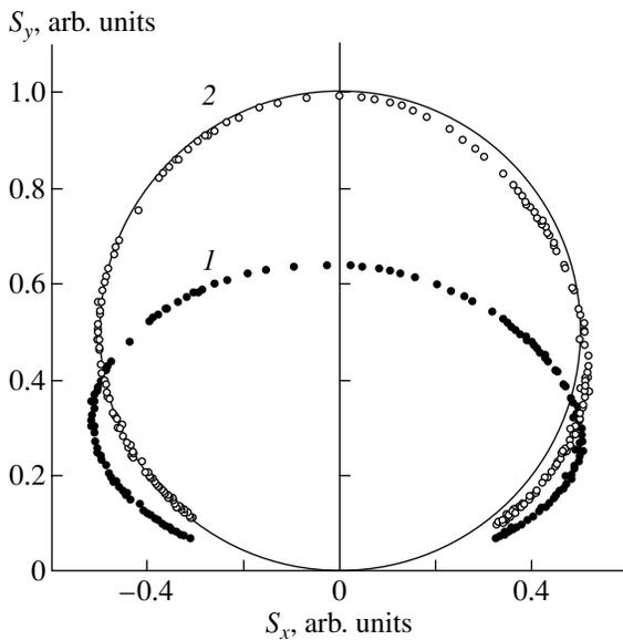
**Fig. 3.** The same record of the  $M_x$  resonance components in a real magnetic field as in Fig. 2 (1) in the laboratory coordinate system and (2) in the natural coordinate system.
