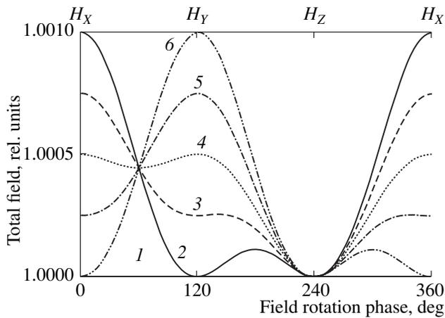
**Fig. 4.** The response of the system to different variations of the  $X$  and  $Y$  components of the measured magnetic field (the plot is normalized to  $H_0$ ): (1) no deviation of the vector, (2) variation of the  $X$  component of the field, (3–5) intermediate cases, and (6) variation of the  $Y$  component of the field.
