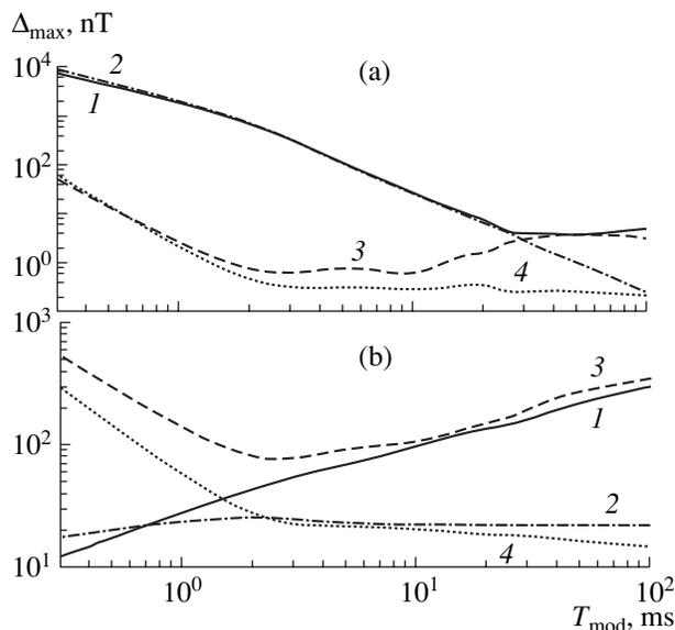
**Fig. 6.** (a) The dependence of the error in the components  $\Delta_{\max} = \max(\Delta_X, \Delta_Y, \Delta_Z)$  for  $\Delta H_X = 10$  nT and  $\Delta H_Y = \Delta H_Z = 0$  on the modulation period  $T_{\text{mod}}$ ; (b) the dependence of the short-term (0.1 s) sensitivity  $\sigma_X$  in the X component on the modulation period  $T_{\text{mod}}$  (1) 1A, (2) 2A, (3) 1B, and (4) 2B.
