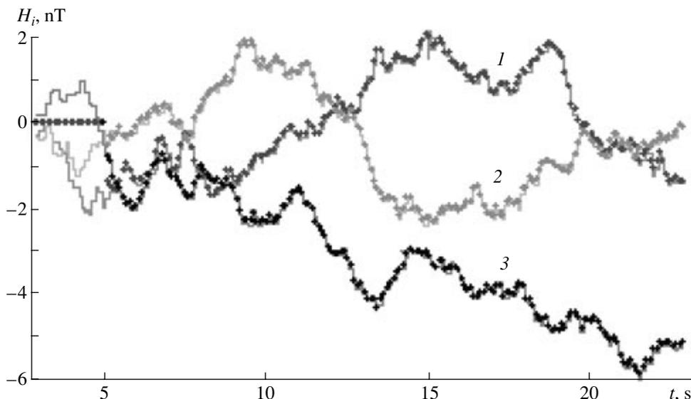
**Fig. 5.** Numerical simulation of the phase-locking process and measurements of the three components of the drifting magnetic field. The solid lines are the components of the measured field; the crosses, measured values of the field. (1)  $H_x$ , (2)  $H_y$ , and (3)  $H_z$ .
