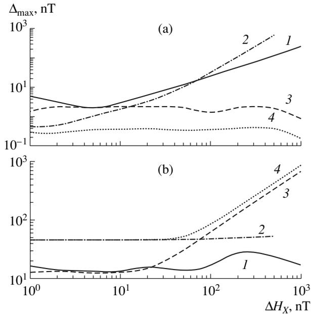
**Fig. 7.** (a) The dependence of the error in the components  $\Delta_{\max} = \max(\Delta_X, \Delta_Y, \Delta_Z)$  on the variation of the field component  $\Delta H_X$  for  $\Delta k_i = 0$ ; (b) the dependence of the error increment in the components on the variation of the field component  $\Delta H_X$  in the case of variation of the coefficient  $k_X$  of the X coils by the value  $\Delta k_X = 0.001$  for  $\Delta k_Y = \Delta k_Z = 0$ . (1) 1A, (2) 2A, (3) 1B, and (4) 2B.
