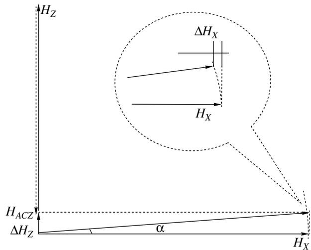
Fig. 2. The error of measuring the  $H_X$  component of the field related to inaccuracy in compensating the  $H_Z$  component.  $\Delta H_Z$  is the residual field along the Z axis and  $\Delta H_X$  is the error of measuring the component  $H_X$ .
