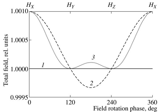
Fig. 3. The dependence of the modulus of the total magnetic field vector on the rotation angle (the plot is normalized to  $H_0$ ): (1) for the direction of the measured field coincident with the axis of the system ( $\Delta H_i = 0, \Delta H_{Mi} = 0$ ), (2) for the variation of the X component of the measured magnetic field ( $\Delta H_X = 1.001, \Delta H_{MX} = 0$ ), and (3) for the variation worked out by the feedback system ( $\Delta H_X = 1.001, \Delta H_{MX} = 1.001$ ).
