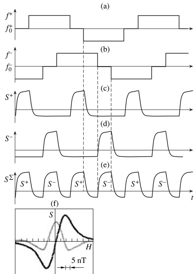
**Fig. 2.** Time waveforms of (a, b) modulation of resonance microwave fields, (c, d) respective signals at the center of the resonance lines, and (e) the net signal at locking of both channels. (f) Shows the resonance signal in one channel at the first and second modulation harmonics.
