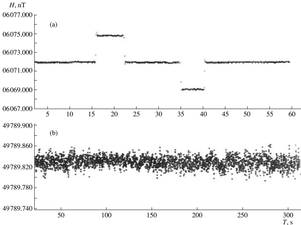
**Fig. 3.** Records made with the HFS magnetometer (10 cps). (a) Field recorded in the screen: the response of the device to a step change in the field and (b) field recorded in the stabilizer. The vertical scale is 20 pT/div.
