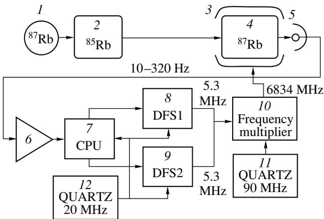
**Fig. 1.** Schematic of the HFS magnetometer: (1) lamp with  $^{87}\text{Rb}$  vapor, (2) isotope filter, (3) microwave cavity, (4) cell, (5) photodetector, (6) photocurrent amplifier, (7) central processor unit, (8, 9) digital frequency synthesizers, (11) high-stability 90-MHz reference oscillator, and (12) 20-MHz reference oscillator.
